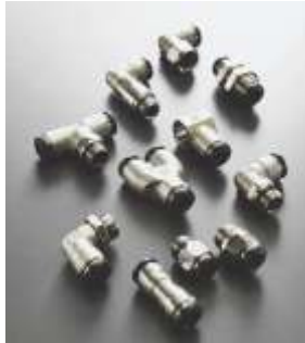
55000 Series with black Collet Push-In Fittings Temp.: -20°C to +80°C Press.: -0.99 bar to 20 bar Fluids: Compressed Air, Vacuum
