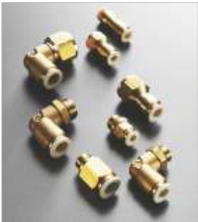
Food & Drink Series Materials: CW510L Brass Body Temp.: -15°C to +190°C Press.: -0.99 bar to 20 bar Specially For Drinking Water & Coffee Machines.
