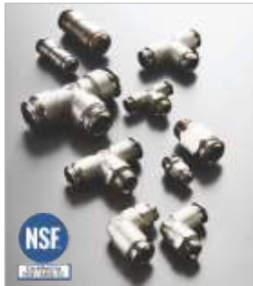
70000 Series Certified Food Grade Push-In Fittings Materials: Nickel Plated Brass Temp.: -15°C to +200°C Press.: -0.99 bar to 20 bar
