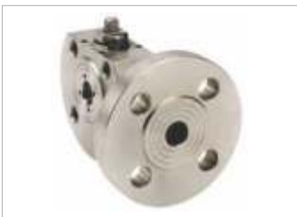
Ball Valve with Free Shafts Material: CS&SS (Temp 10 to 150°C) Ports: 'L' Size Range: 1/2"-4" Pressure Range: PN16,40
