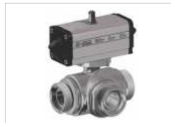
Ball Valve Male Threaded End with DA Actuator Material: SS Ports: 'L' & 'T' Size Range: 3/8"-4" (M&F) Pressure Range: PN16,25,40
