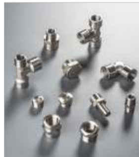
Materials: AISI 316L Max Temp.: -110°C to +300°C Fluids: compressed air, water, oil Max Press.: -0.99 to 140 bar Avail. Sizes: 1/8" to 1"
