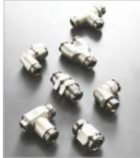
57000 Series Metallic Push-In Fittings Press.: -0.99 bar to 20 bar Temp.: -20°C to +80°C Fluids: Compressed air, Vacuum, Water, Steam (EPDM seal)
