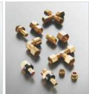
13000 Series (Universal Fittings) Materials: Brass Max. Press.: 148.4 bar Temp.: -60°C to +300°C Avail. Tube Size: 4 - 22 mm
