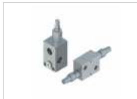
Relief Valves Cartridge and Block type Flow Rate 1 to 180 lpm Max : Pressure 350 bar
