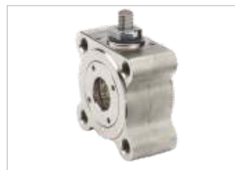
Flat Body Flanged Ball Valve Material: Brass Size Range: 1/2"-2" Pressure Range: PN16
