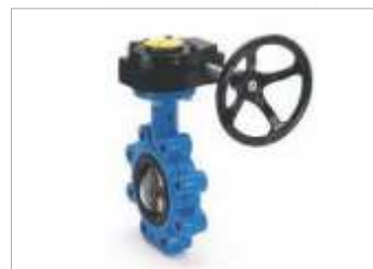
Butterfly Valve with Gear Box (Lug Type) Material: Cast Iron Size Range: 1-1/2" - 12" Pressure Range: PN10/16
