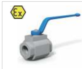
2/2 way ball valve for Gas with Threaded connection (Actuation with one handle) Pmax: 250-500 Bar Size: DN 4-50
