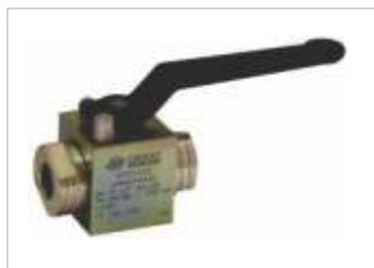
High Pressure Ball Valve with Hand Lever Material: CS & SS Size Range: 1/8"-2" Pressure Range: PN 500
