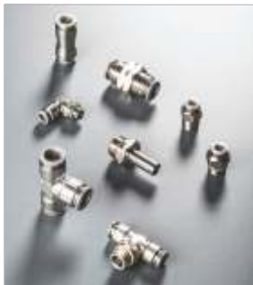
INOX 60000 Series Stainless Steel Push-In Fittings Specially for Food, Chemical Industry Materials: AISI 316L Press.: -0.99 bar to 20 bar Temp.: -15°C to +200°C
