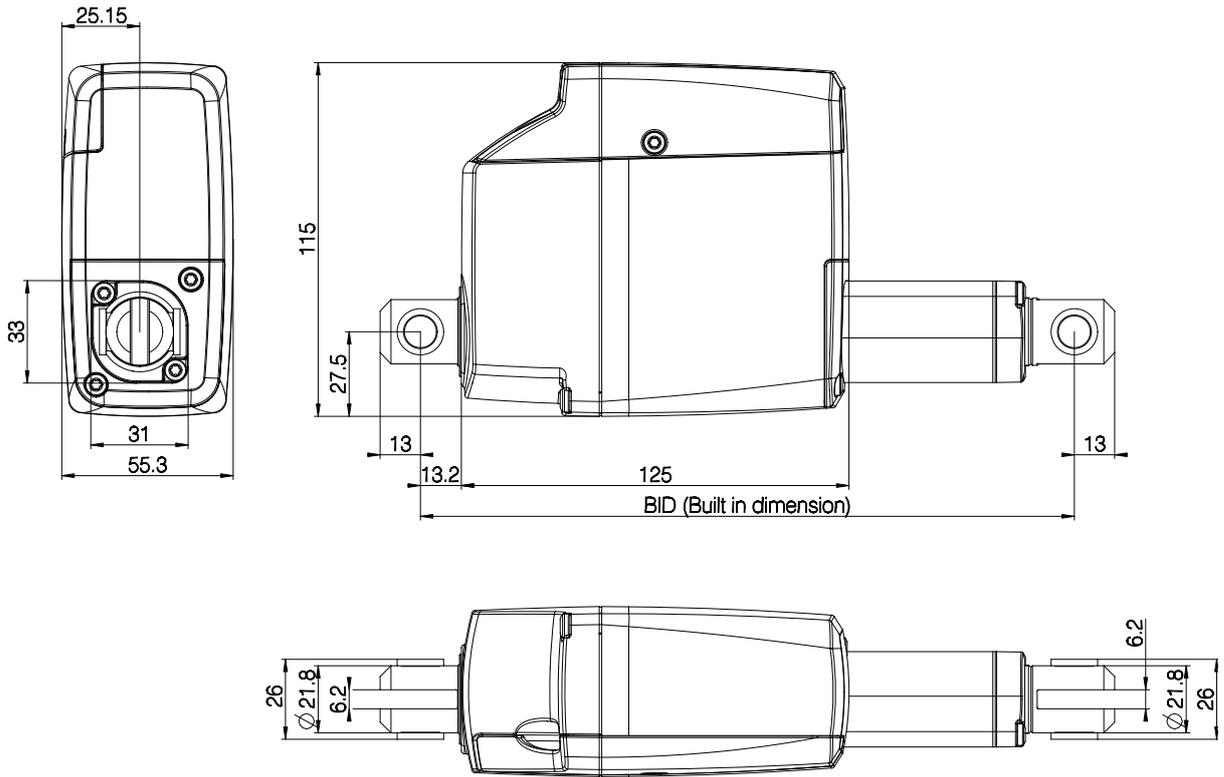
The built-in dimension depends upon the chosen safety option and stroke length (s).
