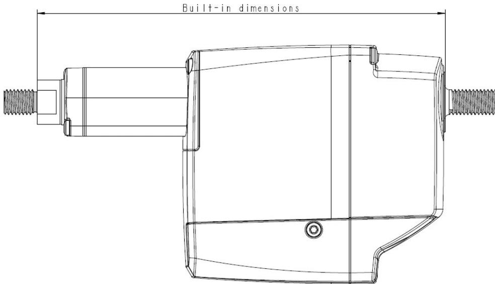
The built-in dimensions for options M and F are measured according to this illustration.
